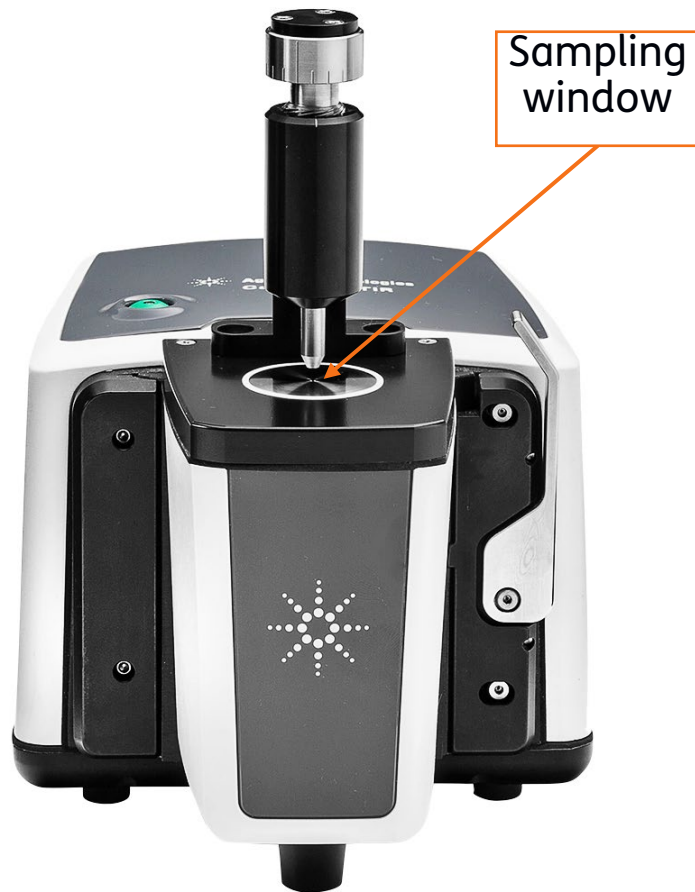
The Mini ATR which is the heart of the online monitoring system
