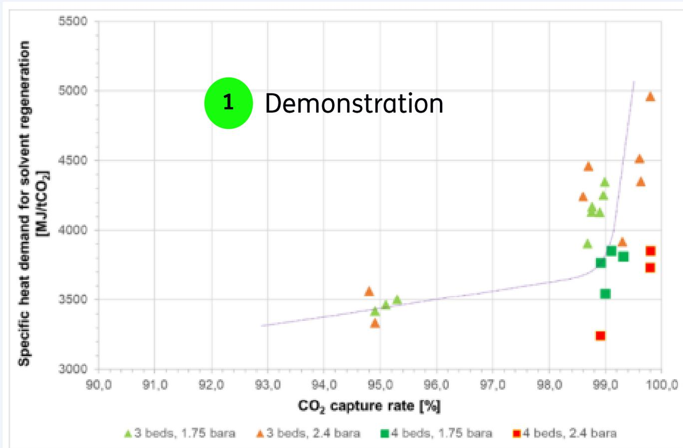
[Demonstration of Highest Capture Rates for Deep Removal - Pilot Plant Test with CO<sub>2</sub> Capture Rates from 98% to >99.9% with an AMP/PZ-Based Solvent by Peter Moser, Georg Wiechers, Peter van Os, Roberta Veronezi Figueiredo, Diego Pinto :: SSRN](#)
