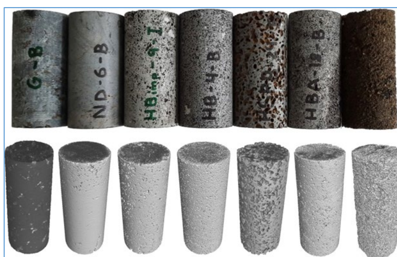
Figure WP1.12: Sample cylinders as used for the experiments. Micro CT scans visualization images (bottom) and reference sample picture (top.)
