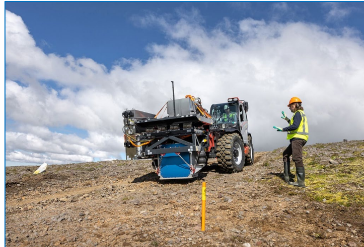
Figure WP4.9: 10kN eVibe during 2022 Iceland survey
