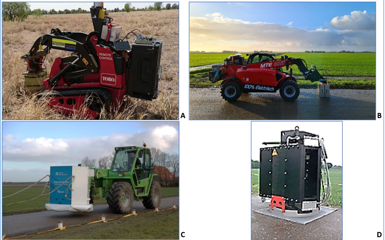
Figure WP4.2: A. The Lightning eVibe, B. The Synchro eVibe, C. 7kN prototype eVibe, D. Linear-motor based vibrator 7kN (TU Delft, Seismic Mechatronics)
