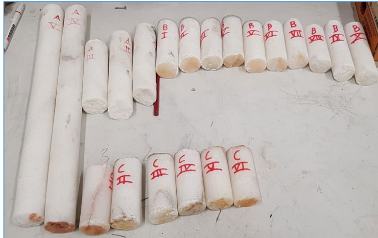
Figure WP3.12: Example. Various core dimensions, for rock mechanics and geochemical experiments by DUT, ICL and METU.
