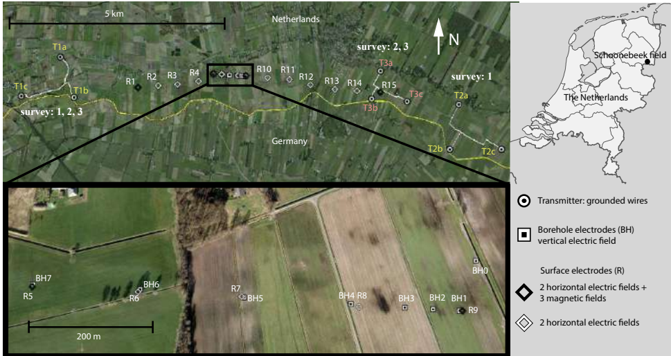
Figure 5.10: Location of field survey and detailed survey layout. Surface electric field receivers are oriented in the north-south and west-east direction. Transmitters are located west and east of the receiver line. Transmitter 1 west of the receiver line is used for all surveys. Transmitter 2 was shifted to location T3 after the first survey.
