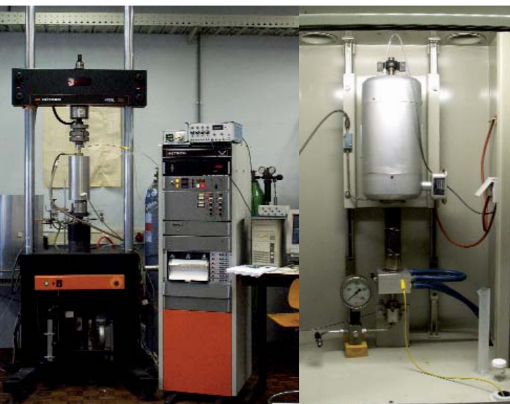
Figure 3.5 Instron set-up (left) and Tuttle bomb set-up (right).
