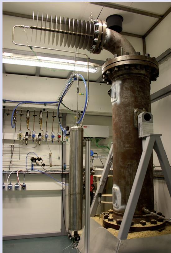
| In this packed-bed reactor, experiments on the reactor scale at elevated pressures (up to 10 bar) will be executed. Picture TUE.
