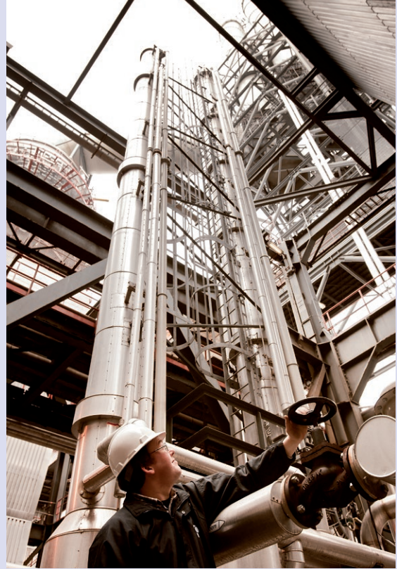
| CO 2 Catcher at the E.ON power plant on the Maasvlakte (near Rotterdam). Picture TNO.
