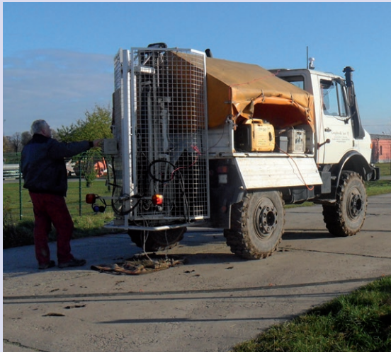
| Active seismic data acquisition at the Ketzin CO 2 storage site. Picture TNO.
