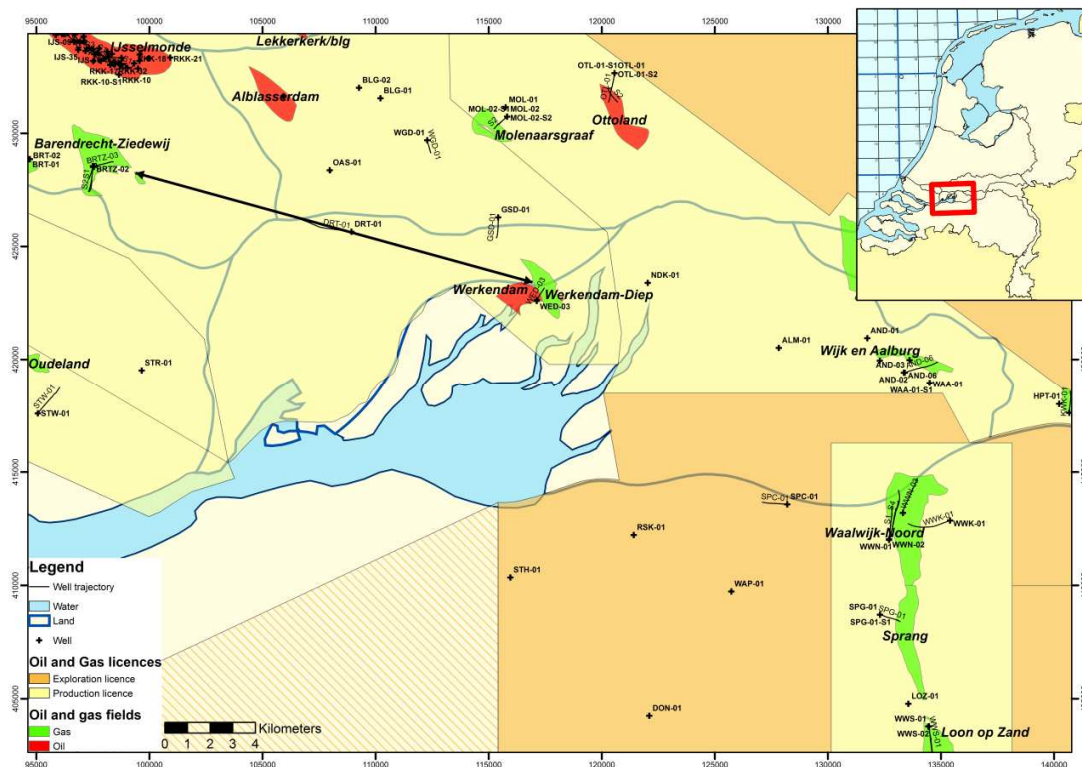
Figure 1. Location of the Werkendam and Barendrecht-Ziedewij gas fields. The Werkendam aquifer is Southwest of, and adjacent to the Werkendam gas field.
