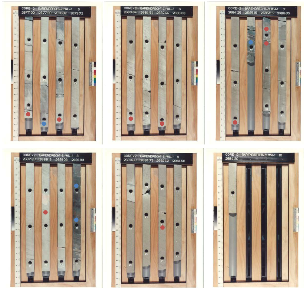
Figure 37. Photos of BRTZ Röt Fringe Sandstone Member (CO 4 reservoir) core and locations of samples. The red dots represent the sandstone samples used in this study. The blue dots represent clayish samples.
