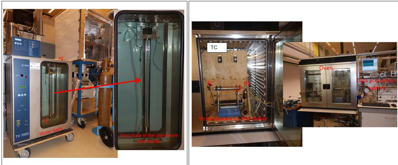
Figure 20. The experimental set up for CO 2 sorption experiments.
