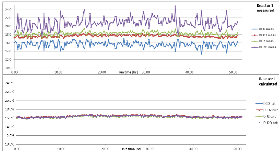
Figure 4-13: Reactor 1 \Delta CO , \Delta H_2O , -\Delta CO_2 and -\Delta H_2 for directly measured values (top) and the calculated values based on the measured dry gas components (bottom)
