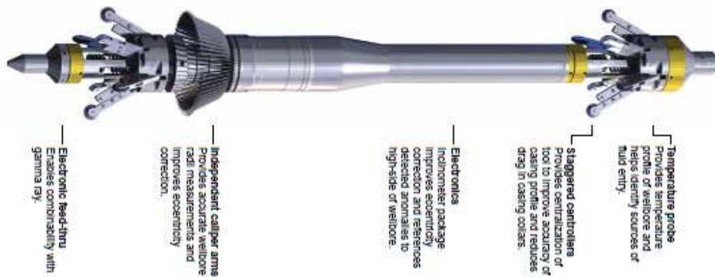
Figure 6-2. An example of a multifinger caliper tool. This particular tool is also capable of temperature measurement. Localised temperature anomalies are an indication of casing leaks, and temperature measurements are used for leak detection regularly (Weatherford, 2010a).
