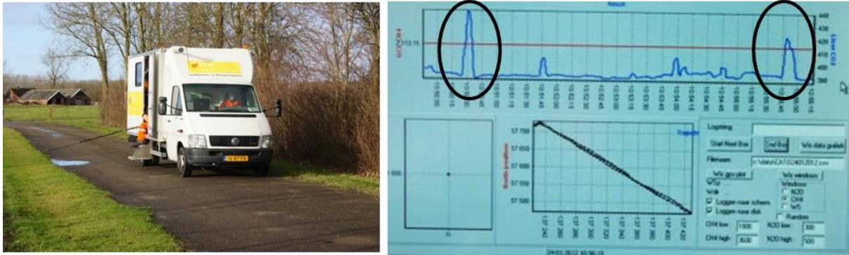
Figure 4.4 mobile CO<sub>2</sub> and CH<sub>4</sub> plume measurements around the Ten Post site.
