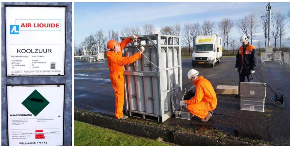
Figure 3.4 : Artificial release experiment installation at the Ten Post site
