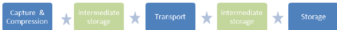
Figure 6. Simplified over illustration of elements (boxes) and the interfaces (stars) in the Carbon Capture and Storage chain. Note that intermediate storage elements are optional
