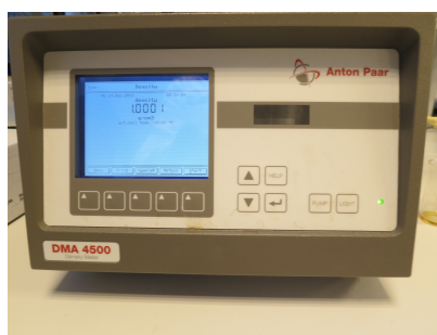
Figure B-1: The used device for the measurement of the solvent density
