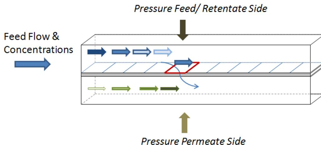
**Figure 3.** Schematic representation of the working mechanism of the membrane separation performance model. The horizontal segmented plane in the middle represents the membrane. For each slice, based on the local concentration of components in the gas stream on both sides, sequentially new concentrations and permeation are calculated.
