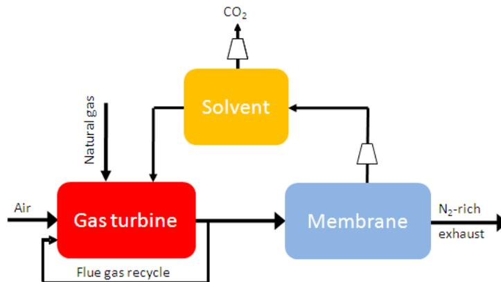
**Figure 1.** The concept of hybrid membrane-absorber CO<sub>2</sub> capture from gas-combusted flue gas
