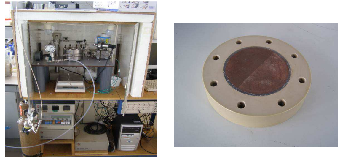
Figure 2 a & b: Capillary pressure setup and to be investigated shale sample.
