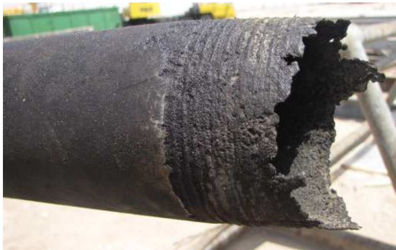
Figure 4.2. A pin and box coupling failure due to H 2 S gas (1000 ppm) + 2% CO 2 .
