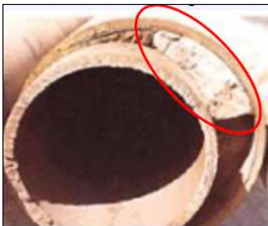
Figure 4.9. Left: unevenly distributed cement (circled) due to eccentric casing (courtesy Schlumberger). Right: mud channel (red) in inclined well.
