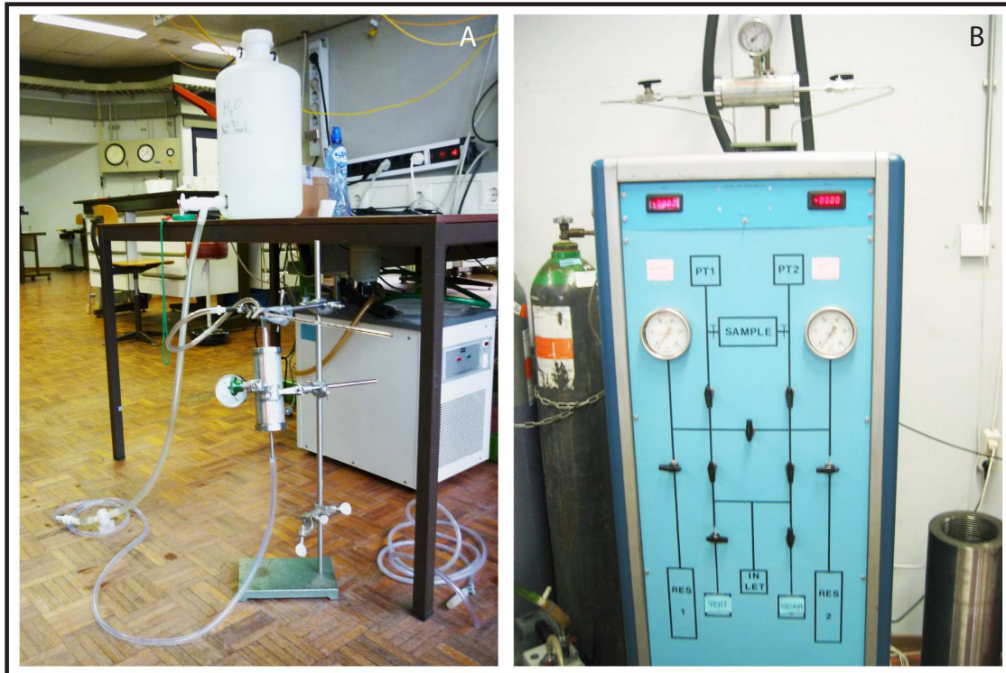
Fig. 10: Photos of (A) the set-up used for (quasi)-constant-head, steady-state H 2 O flow-through permeametry and (B) the Argon permeability apparatus, used for the transient step method. Both methods are applied to determine the permeability of P18 reservoir- and Eiffel samples of Main Bunter sandstone rocks. The steady state flow-through measurements were performed at different head lengths to confirm reproducibility of the dataset. Head lengths were varied from 0.2 to 2.2 m, corresponding to pressure gradients of ~2 to ~20 kPa. Similarly, for the transient step measurements we varied the mean upstream/ downstream pressure between 1.5, 1 and 0.5 MPa, keeping the (initial) differential pressure at 0.2 MPa.
