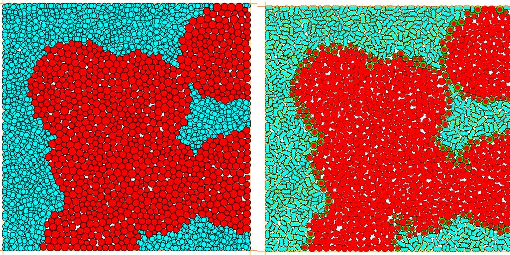
**Figure 1.** Discrete element model of anhydrite caprock before reaction with CO<sub>2</sub> (left) and after 50000 years exposure to CO<sub>2</sub>-rich fluids. Matrix anhydrite grains (blue), anhydrite rosettes (red), reaction rims of calcite in matrix grains (yellow) and rosettes (green) are indicated.
