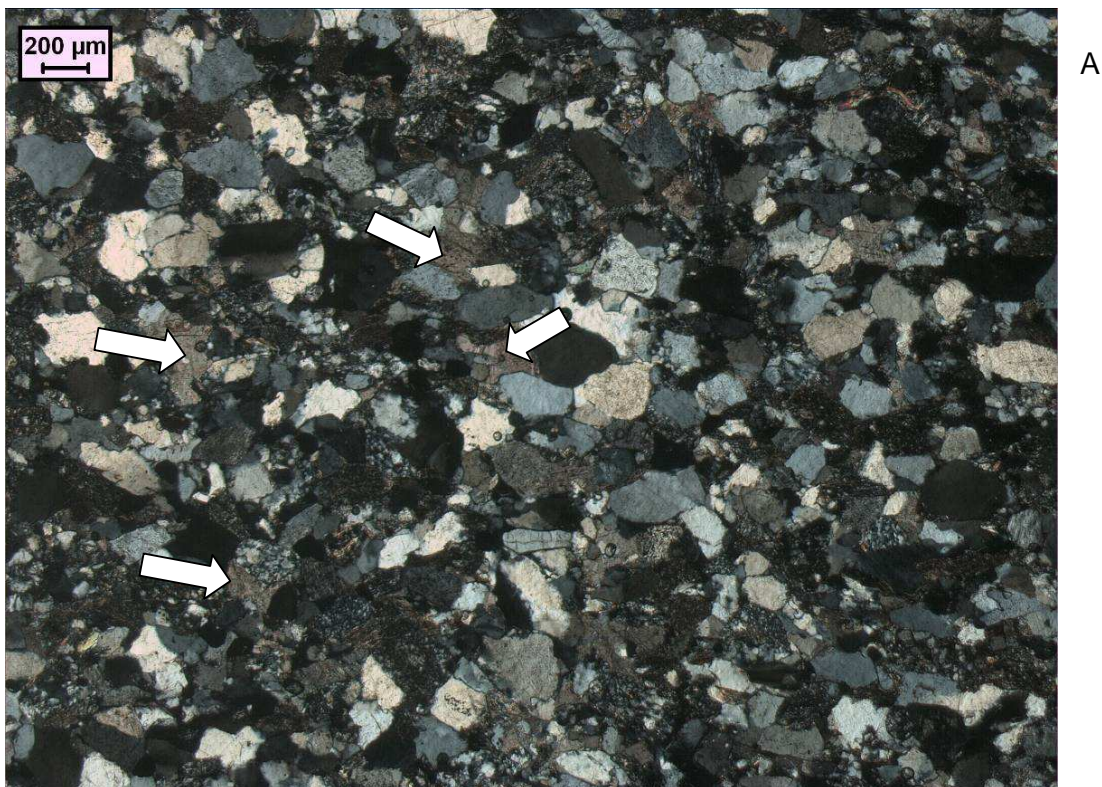
Figure 11: Volpriehausen sst. A) Sample 4b, crossed polarized light. White arrows show areas of calcite cement.
