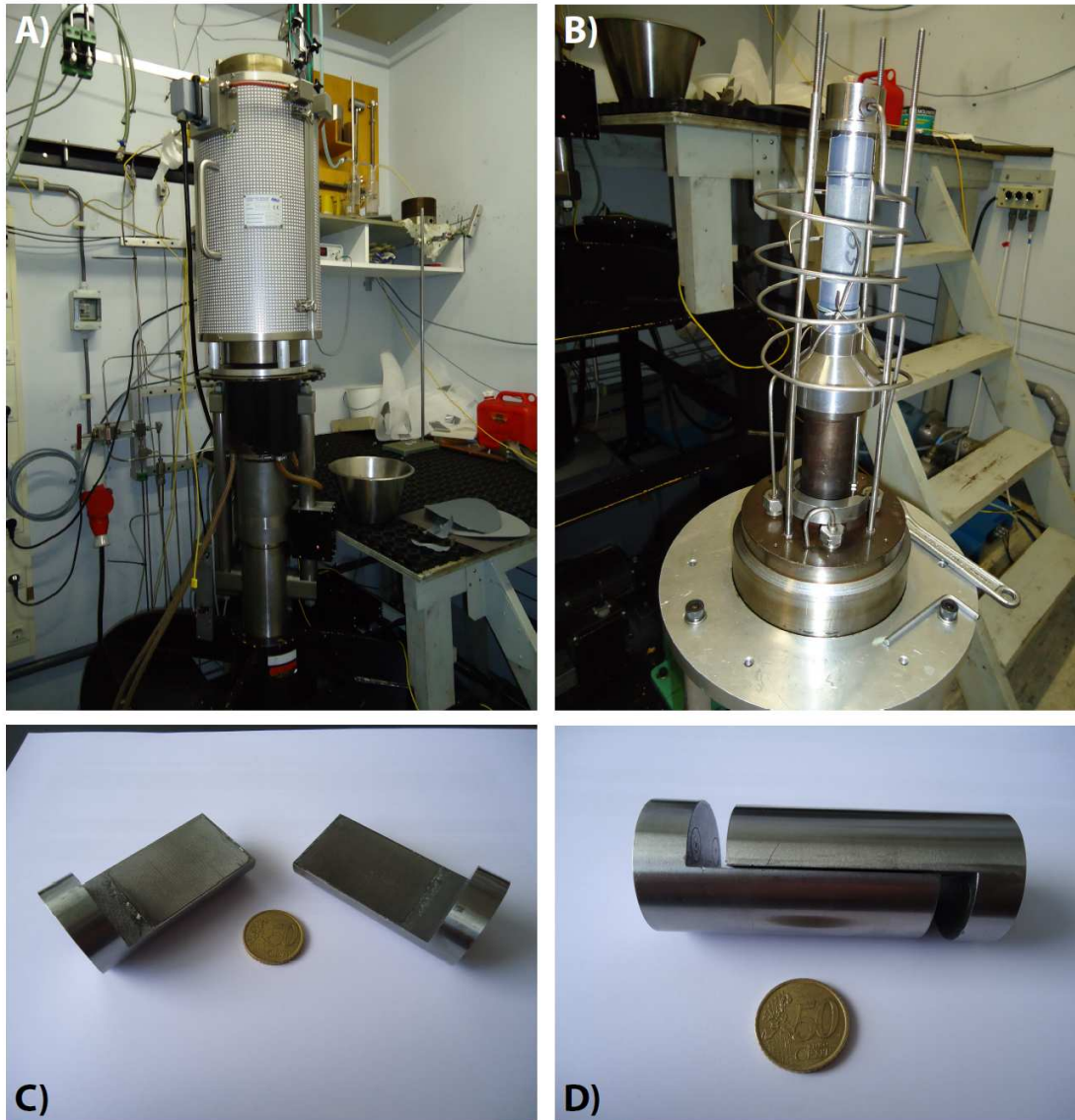
Figure 1 - The Heard Apparatus is a constant confining volume triaxial pressure vessel capable of generating 100 MPa confining pressure at temperatures of up to approximately 250 °C using EPDM and FEP jacketing materials. A) The Heard vessel is surrounded by an external furnace (silver) and is loaded vertically from the bottom of the pressure cell. Temperature is monitored internally, in contact with the experimental sample as well as externally. B) The sample is held in place inside of a heads-piece which is inverted, slid into the top of the Heard vessel, and sealed using o-rings, and a steel on steel cone style connection. Sample shown here is a 25mm diameter rock core, ~60mm in length (UU-Sample I.D.: 55). C) 35mm diameter forcing blocks for “inverted-shear” style direct shear in the Heard apparatus (50 euro cent piece for scale). Both sides of the inverted-shear geometry are fitted with 33 x 47 mm sintered porous steel fluid distribution plates. D) inverted-shear blocks fitted together in experimental configuration, will be placed into the heads-piece in the same configuration as the rock sample in B)
