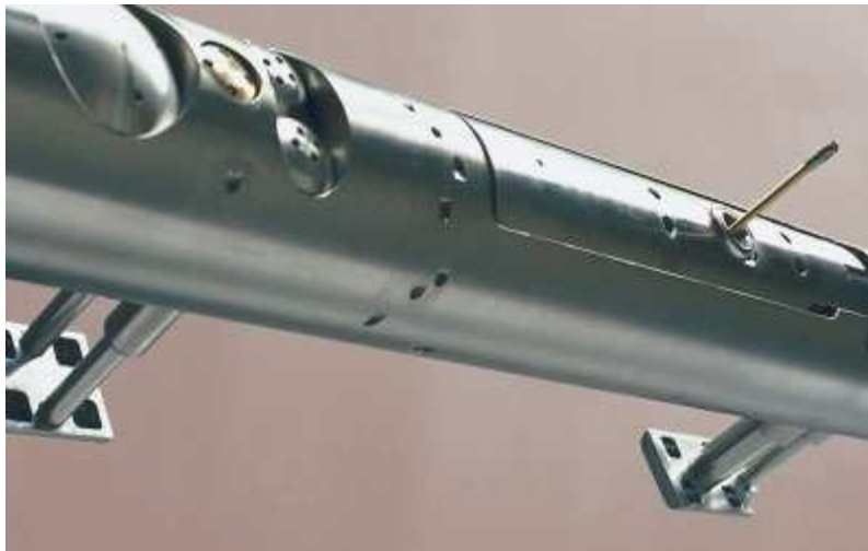
Figure 3: The cased hole dynamic tester (CHDT) (Source: Schlumberger)
