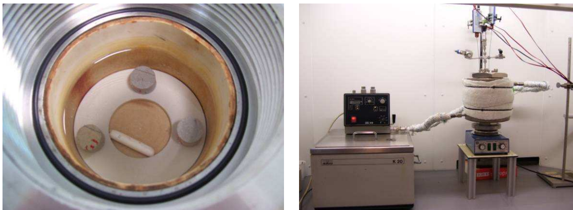
Figure 10 - Left: Pressure vessel and Teflon reservoir containing 3 small cement samples, brine and a stirring device. Right: Experimental setup with the heat bath on the left and the vessel on the right, isolated by glass wool. Thermocouples and pressure measurement devices are placed on the cover of the pressure vessel and attached to a computer to monitor pressure and temperature of the brine and the supercritical CO 2 during the experiments.
