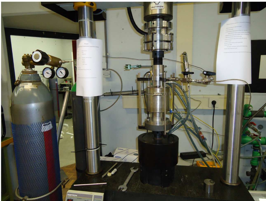
Figure 9 - Force of crystallization experiments are conducted in a reaction vessel fitted into an Instron load frame. A small sample of a combination of powdered caprock, cement, and ground N80 steel is pressurized with supercritical CO 2 and allowed to react under a small constant vertical load. As the sample swells due to reaction with CO 2 over the course of the experiment, the load frame will retract in order to maintain the set vertical load. By measuring the change in volume of the sample we are able to calculate a so-called force of crystallization, which may be of significant importance in potentially fracturing the caprock, leading to loss of containment of the CO 2 reservoir.
