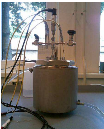
Fig. 12: The HPT vessel used for the corrosion experiments.
