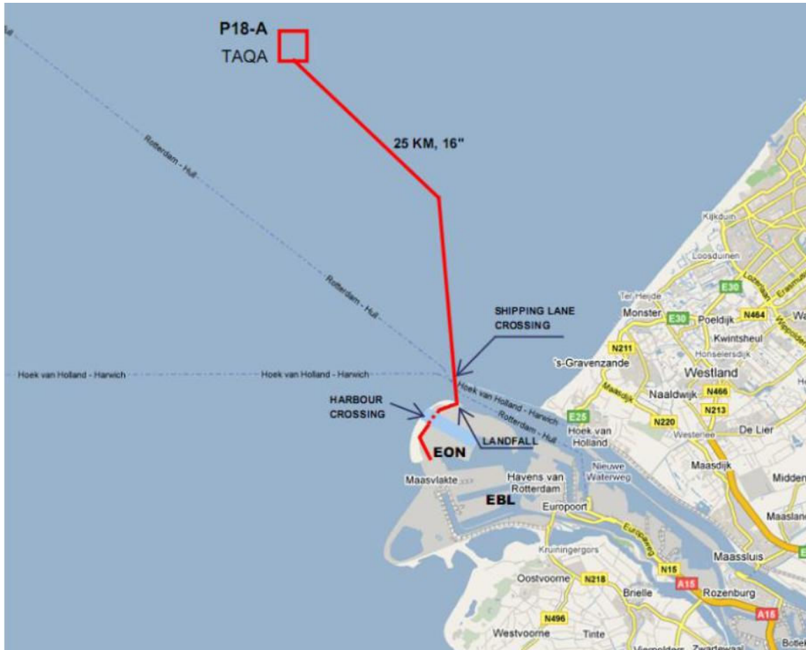
Figure 4.6 Location of E.On's new coal power plant and routing of CO 2 transport (Source: GdF Suez, 2010) 4
