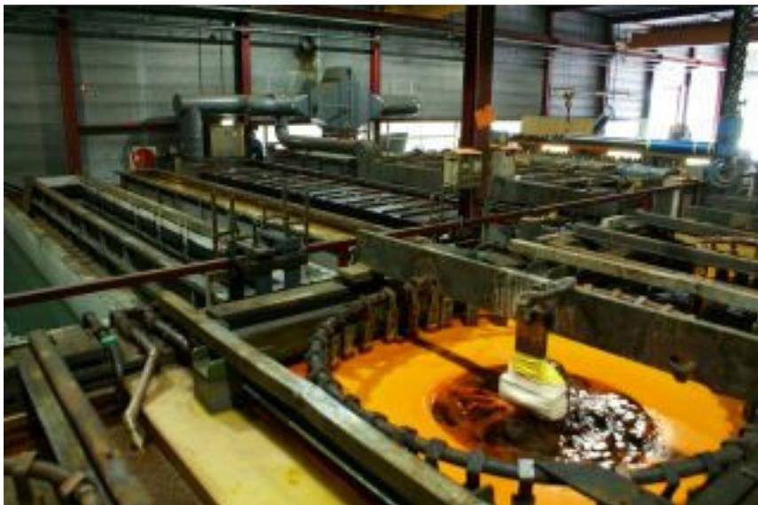
Figure 5.1 *Example of large scale chromium plating bath at Technochroom/DMI*
