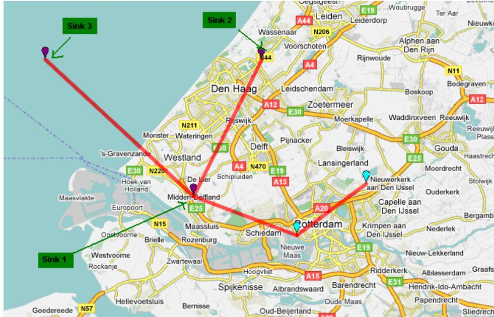
Figure 8. Pipelines network computed by the network algorithm
