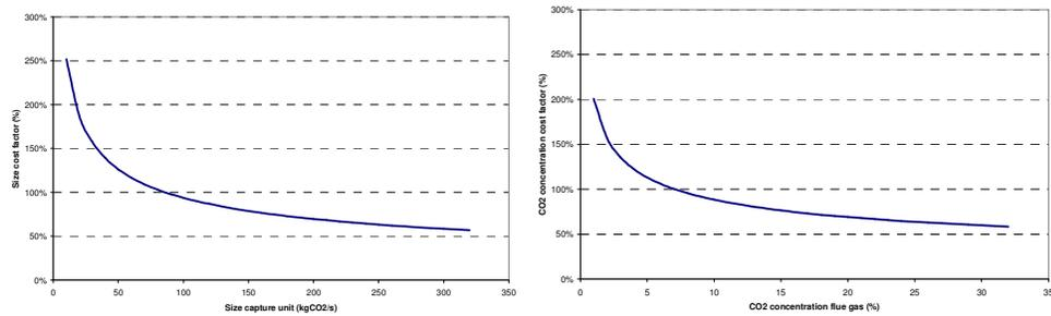
Figure 6. Relationship between capture unit size and relative specific capital costs (left figure), and relationship between CO<sub>2</sub> concentration in flue gas and relative specific capital costs (right figure)
