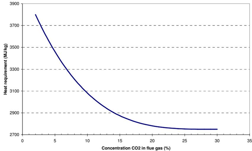
Figure 5. Heat requirement fit for amine-based capture process of carbon dioxide from flue gases for maximum heat integrated systems
