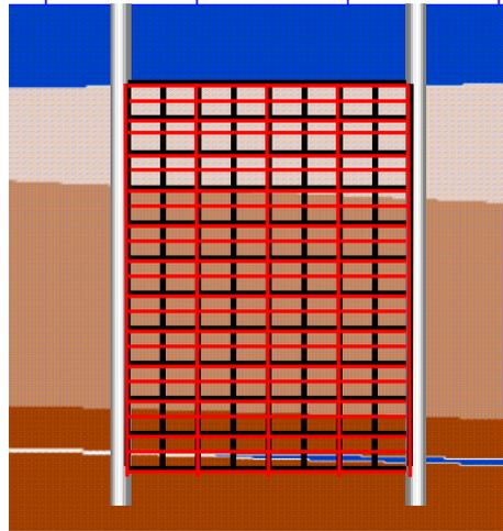
*Figure 4: Grid parameterisation of the subsurface model: definition of a squared grid (black) and a rectangular grid (red) to be used for tomographic inversion between the wells. Only for demonstration purposes very coarse grids are displayed. As a result of the inversion seismic velocities (or seismic amplitudes) are allocated to the grid cells.*
