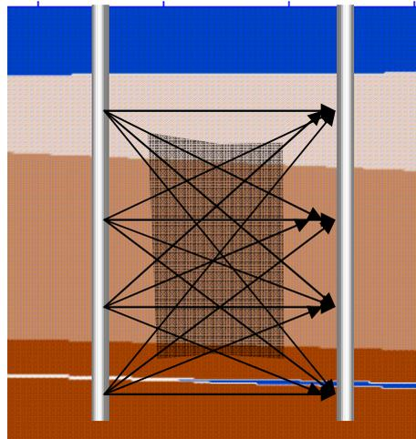
*Figure 1: Example of a subsurface model with two vertical wells. The sources are positioned in the left well; the receivers are positioned in the right well. Possible ray paths of direct waves are drawn from 4 source positions to 4 receiver positions. As can be derived from the ray path density, the indicated grey area between the wells is best sampled. The areas below the lowest positions, above the top positions and near the wells are less well defined.*
