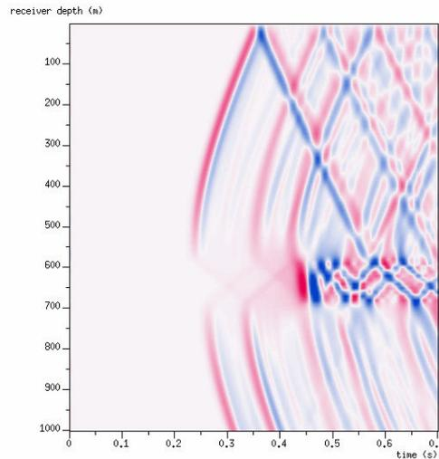
*Figure 5: Example of synthetic modelled data showing crosswell arrival times. A low velocity interval is present at 600-700 m depth (Winthagen, 2005). The travel paths through the low velocity layer arrive at about 0.45 s. Note the bow-tie structures in this low-velocity interval that correspond to travel paths through surrounding layers.*
