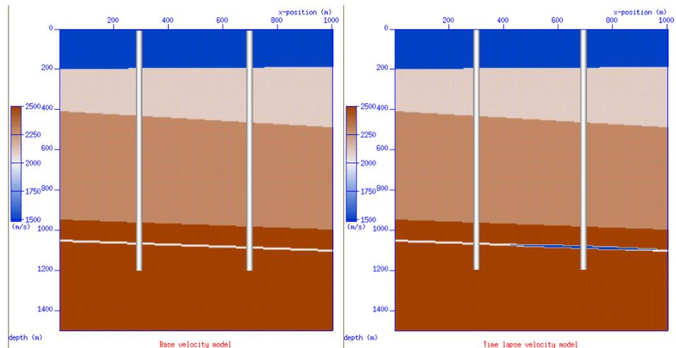
Figure 2: A seismic velocity-depth model is used to investigate the effect of CO<sub>2</sub> injection to the seismic crosswell response. a) the situation before injection. b) the situation after injection resulting in a reduction of seismic velocity.
