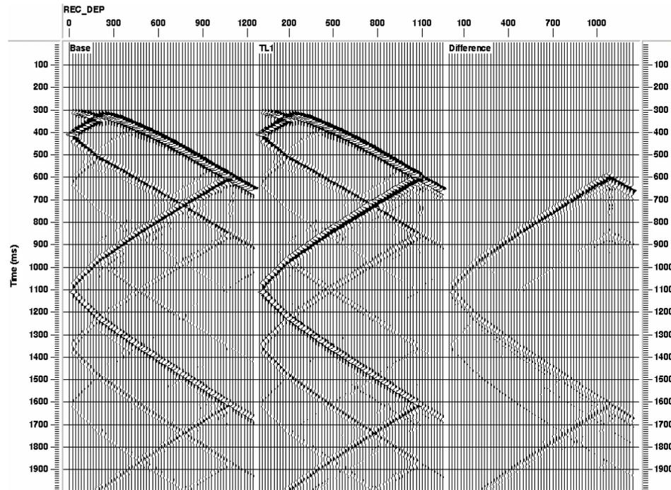
Figure 3: The source is positioned in the left well at a depth of 300 m and the receivers are located in the right well at 0-1250 m depth (x-axis). Shown are the shot gathers prior to (left) and after injection (middle; see also Figure 1). On the right the difference in seismic response is shown.
