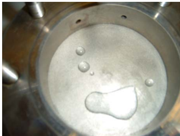
Figure 7 Water breakthrough in the porous plates: hydrophilic patches embedded in a hydrophobic environment
