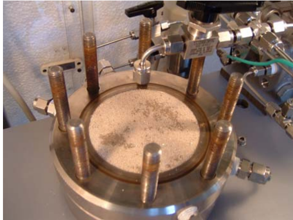
Figure 8 Visualization experiment: water breakthrough in a coarse sand sample
