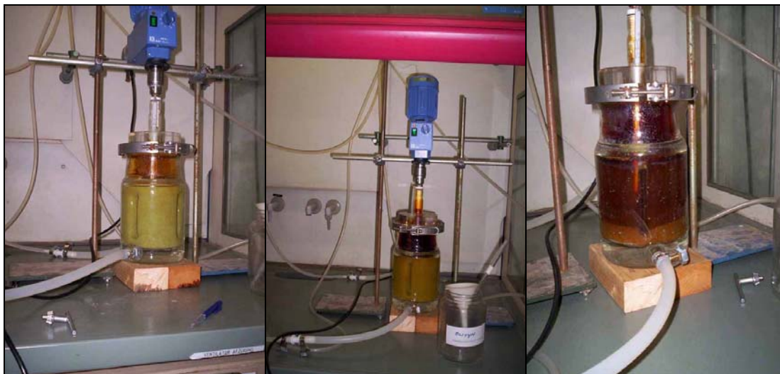
Fig 3.1: Glass reactor from left to right at the beginning of extraction, at the end of extraction and at the end of experiment no 14.
