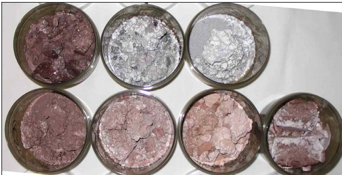
Figure 5.4: Residues from Mg(NO_3)_2 \cdot 6H_2O decomposition tests, top row from left to right: dest 4, 5, 6, bottom from left to right dest 7, 8, 9 and 10.
