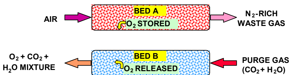
Figure 2.6 O_2 -production by CAR process (Source BOC).
