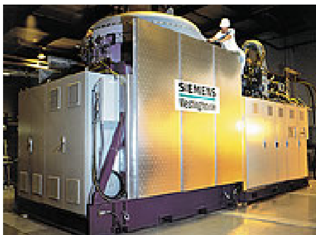
Figure 2.10 SOFC and gas turbine hybrid demonstrator 220 KW at the University of California [Source Siemens internet [31].
