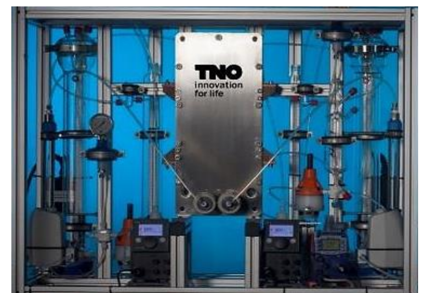
Figure 6 Electrolyser system (1600 cm 2 ) developed at TNO for continuous electrochemical production.
