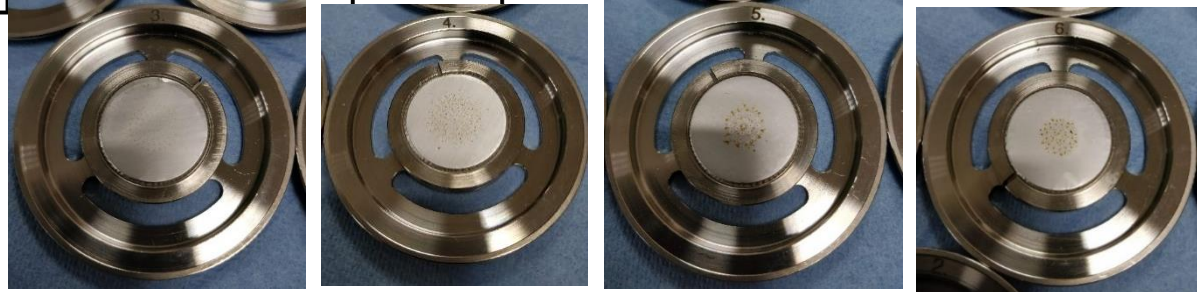
From top left: Stage 3 (0.0265 \mu m), Stage 4(0.0485 \mu m), Stage 5 (0.087 \mu m) and Stage 6 (0.147 \mu m)
